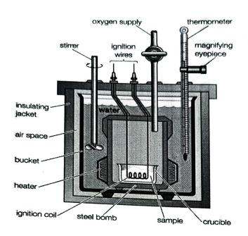
The One Commonly Used for the purpose in the "Atwater" bomb calorimeter. It consists of heavy steel bomb, with platinum (or) gold plated Copper Lining. It has a cover which is held tightly by a strong screw - Collar. A weighed amount of sample & the bomb is charged with an Oxygen Valve. The valve is then closed & the bomb ik immersed in a weighed amount of water.
