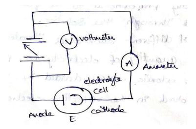
Besides the electrodes, the circuit also requires a. d. c current sources rated at 3-15V, a variable resistance, and an ammeter a voltmeter, a magnetic stirrer and a hot plate. All these components are provided in commercial electrolysis units and a may sometimes include a spinning inner electrode to assist in stirring the solution undergoing electrolysis.
