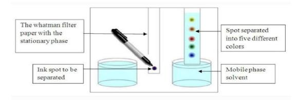
Paper chromatography for the determination, the sample mixture is spotted & the paper by a micro syringe (or) capillary tube, then the paper is introduced into the sample solvent ethylene, solvent is do not tough the application of sample & barbitone is applied on the paper at distance from the sample.
