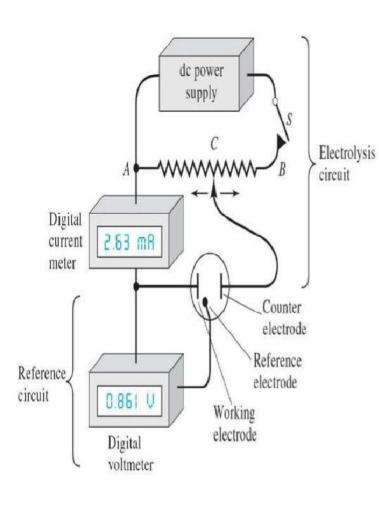
Apparatus for controlledpotential, or potentiostatic, electrolysis. Contact C is adjusted as necessary to maintain the working electrode (cathode in this example) at a constant potential. The current in the reference electrode is essentially zero at all times. Modern potentiostats are fully automatic and frequently computer controlled. The electrode notations in the figure are the currently acceptable notations.
